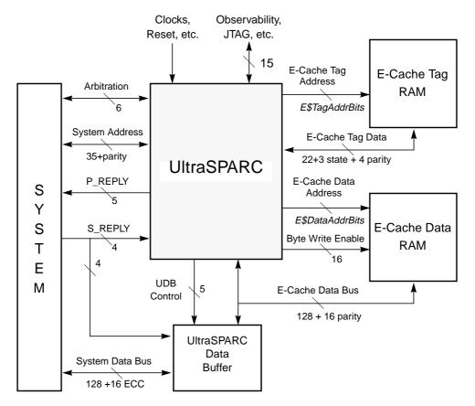
Figure 7-1 Main UltraSPARC Interfaces
