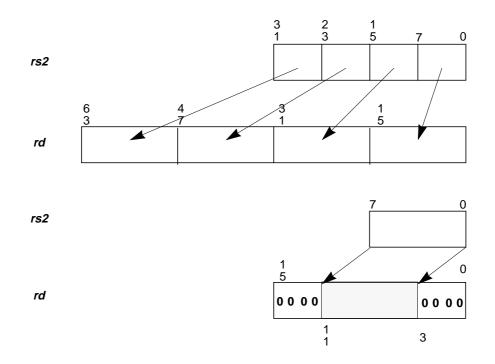
Figure 13-6 FEXPAND Operation
