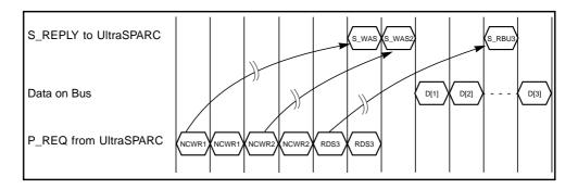
Figure 7-28 S\_REPLY Pipelining to UltraSPARC for Data Transfers
