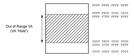
Figure 4-2 UltraSPARC's 44-bit Virtual Address Space, with Hole (Same as Figure 14-2)
