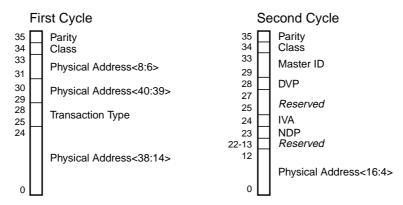
Figure 7-32 Packet Format: Coherent P\_REQ and S\_REQ Transactions
