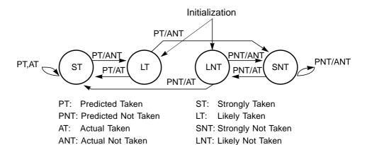
Figure A-15 Dynamic Branch Prediction State Diagram
