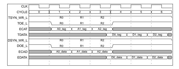
Figure 7-3 Timing for Coherent Read Hit (1–1–1 Mode)
