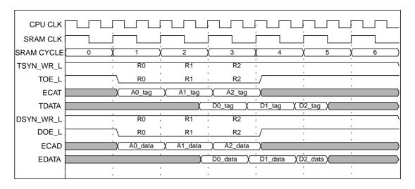
Figure 7-4 Timing for Coherent Read Hit (2–2 Mode)
