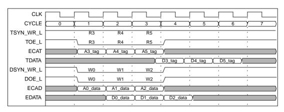
Figure 7-8 Timing Overlap: Tag Access / Data Write for Coherent Writes (1–1–1 Mode)
