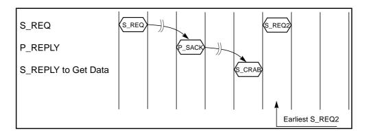
Figure 7-27 Back-to-Back Coherent S\_REQs to UltraSPARC
