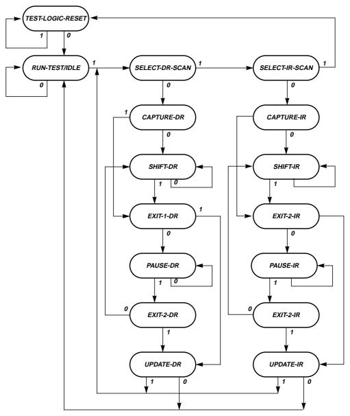
Figure D-1 TAP Controller State Diagram
