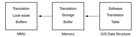
Figure 4-3 Software View of the UltraSPARC MMU
