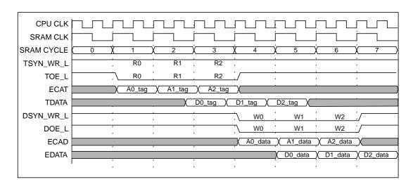
Figure 7-6 Timing for Coherent Write Hit to M State Line (2–2 Mode)
