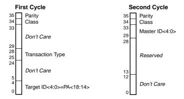
Figure 7-34 Packet Format: P\_INT\_REQ Transaction
