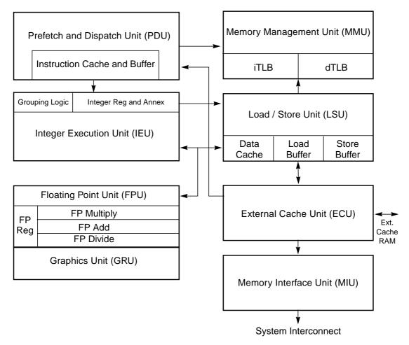
Figure 1-1 UltraSPARC Block Diagram
