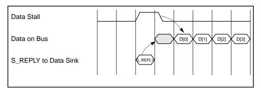
Figure 7-30 Data\_Stall to UltraSPARC Sinking Data
