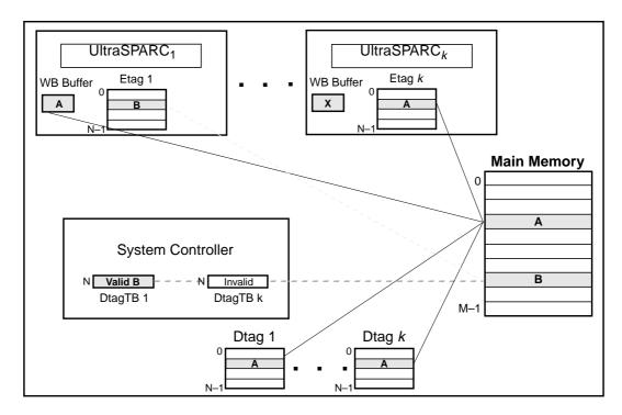
Figure 7-21 Cache Coherence Model Using Centralized Duplicate Tags (Dtags)
