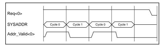
Figure 7-11 Uniprocessor: Back-to-Back Packets—No SC Request
