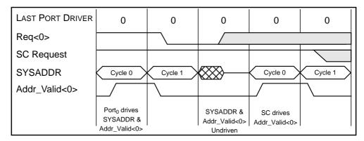
Figure 7-15 Arbitration: SC Arbitrates and Sends a Packet to Port<sub>0</sub>
