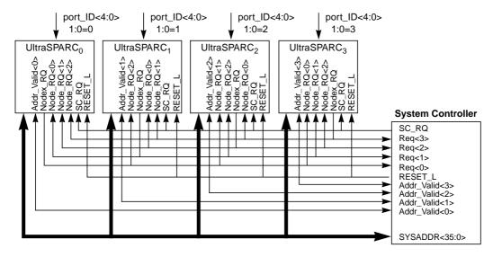
Figure 7-10 SYSADDR Bus Interconnection Topology
