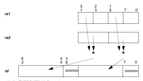
Figure 13-13 FMULD8SUx16 Operation
