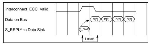
Figure 7-25 S\_REPLY Timing: UltraSPARC Receiving Block Write—No Data Stall
