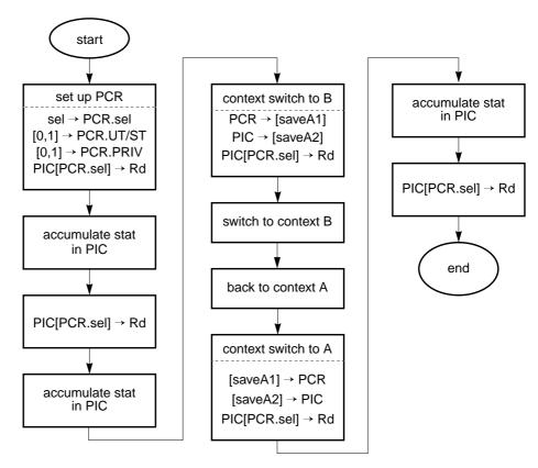
Figure B-3 PCR/PIC Operational Flow
