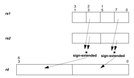
Figure 13-14 FMULD8ULx16 Operation
