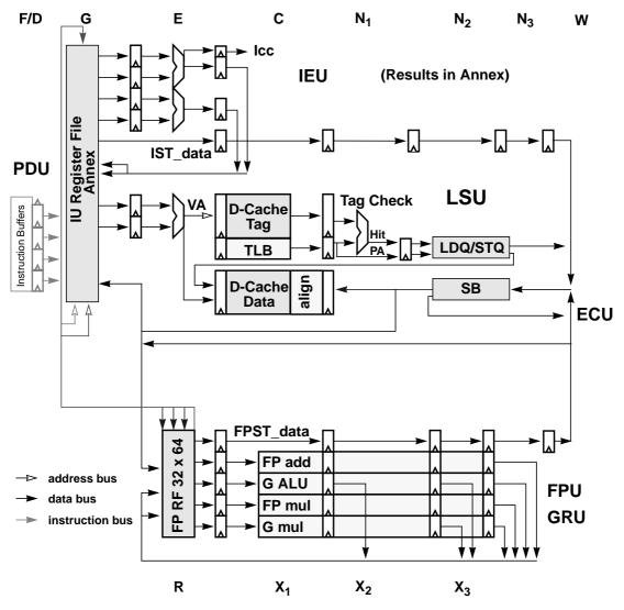
Figure 2-2 UltraSPARC Pipeline Stages (Detail)
