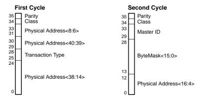
Figure 7-33 Packet Format: Noncached P\_REQ Transactions
