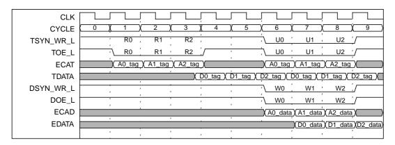
Figure 7-7 Timing for Coherent Writes with E-to-M State Transition (1–1–1 Mode)
