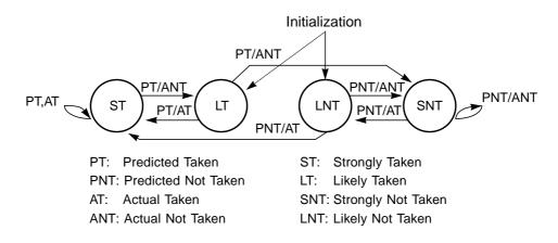
Figure 16-6 Dynamic Branch Prediction State Diagram
