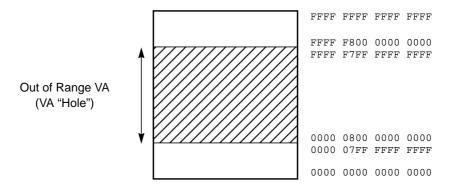
Figure 14-2 UltraSPARC's 44-bit Virtual Address Space, with Hole (Same as Figure 4-2)
