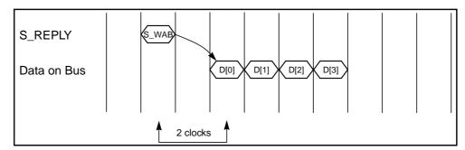
Figure 7-24 S\_REPLY Timing: UltraSPARC Sourcing Block Write—No Data Stall
