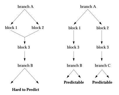
Figure 16-10 Branch Transformation to Reduce Mispredicted Branches
