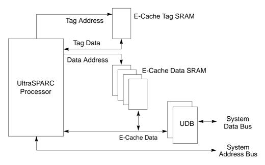
Figure 1-2 UltraSPARC Subsystem
