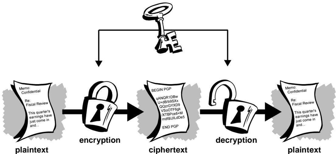
Figure 1-2. Conventional encryption
