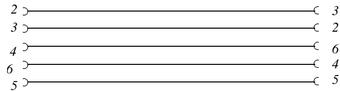
Fig. 9-1: SubD 9-pole (female) to SubD 9-pole (female) (AMU <--> AMU)
