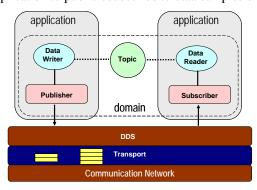
Fig. 1. Architecture of DDS
