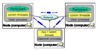
Fig. 4. Centralized DDS Architecture
