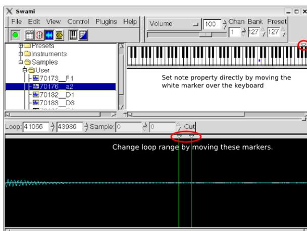
When creating a chromatic instrument from a set of samples that cover different pitch ranges (bass, mids, trebles), further actions need to be done to make sure you get a continuous sound.
